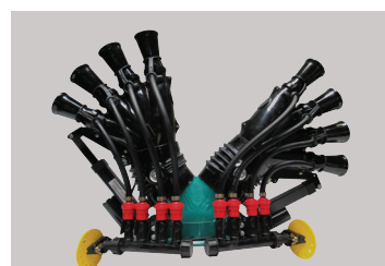
Electro cylinders with control box operated from tractor seat (inner spray heads)
